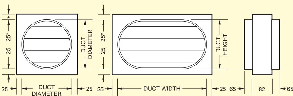
\* + OR - 11mm FROM A 50mm HEIGHT INCREMENT RESULTS IN A 50mm TOP HAT SECTION.
